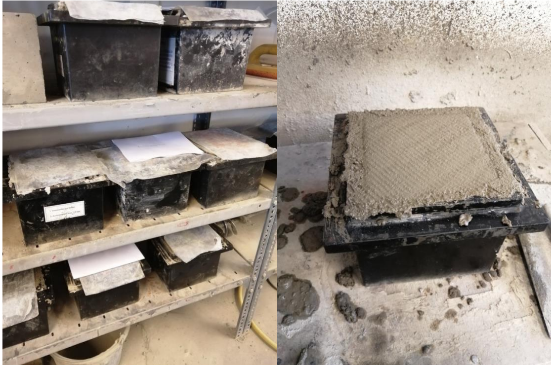
Figure 6. Concrete test cubes drying before water bath
