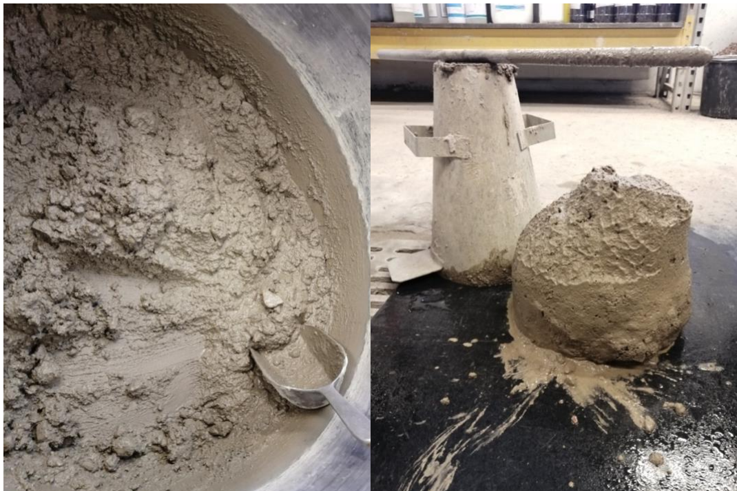
Figure 5. Fresh concrete and a successful 11 cm slump
