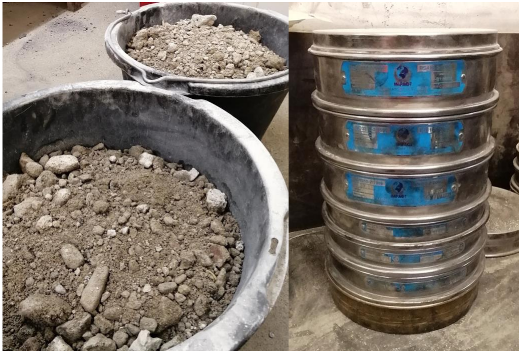
Figure 2. Concrete aggregate before sieving (left) and laboratory sieve set used in the experiment (right)
