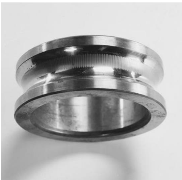
Figure 10. Damaged inner ring of bearing. Noticeable fluting pattern caused by bearing currents. (Ahola J. 2011, 6)
