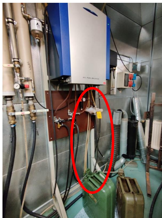
Figure 17. Actual fuel injection equipment signaling the fuel tank inlet fuel white pipes - enclosed in red (Author's own).
