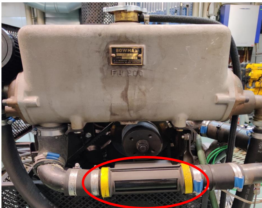
Figure 25. The temperature sensor of the cooling system of the SISU 420 DWI Diesel Engine (Author's own).
