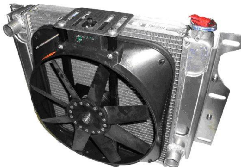
Figure 7. Radiator with a puller fan configuration (Mathworks.com, 2022).
