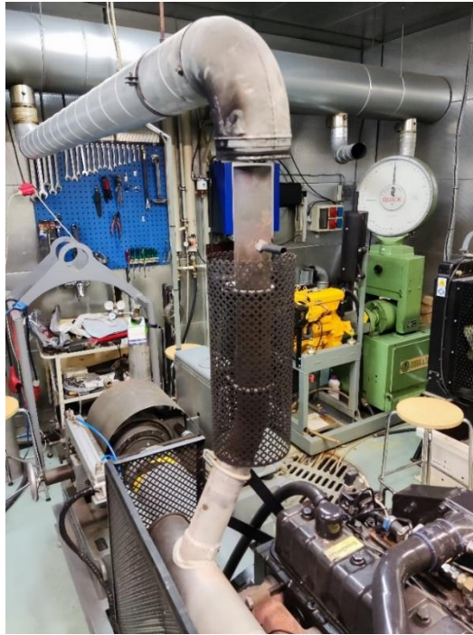
Figure 38. Extractor pipe and tailpipe photo of the laboratory exhaust gas system (Author's own).
