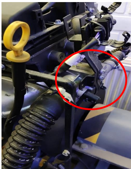
Figure 28. Inlet port of the coolant to the engine block where the thermostat is placed (Author's own).
