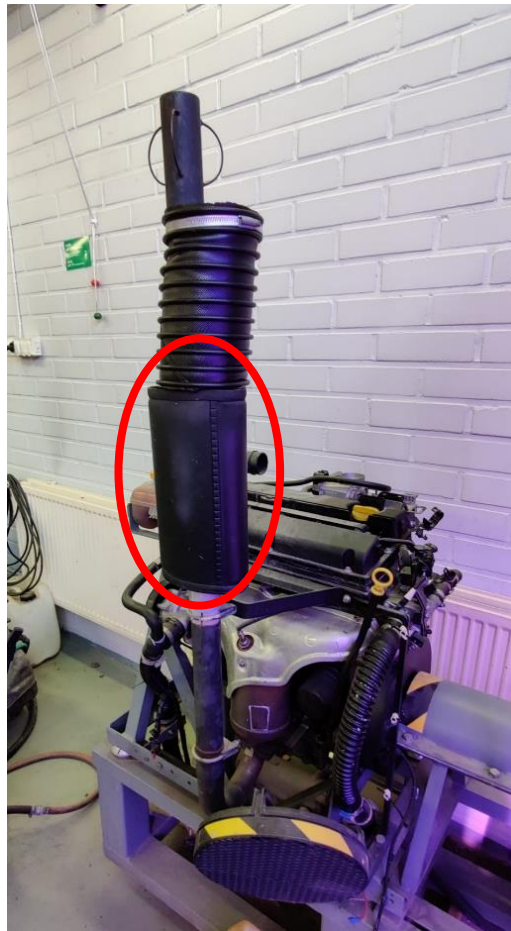
Figure 37. Display of the Opel's engine exhaust muffler (Author's own).
