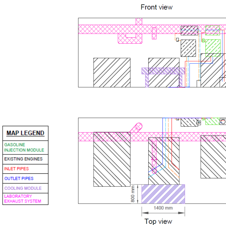
Figure 100. Final installation scheme (Author's own).
