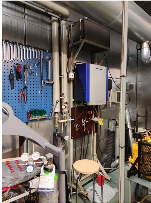
Figure 16. Diesel injection system. From down to up, the fuel consumption device (blue and grey box), the pre-filter (left-hand side of the fuel measurement item and the fuel tank (grey box) (Author's own).
