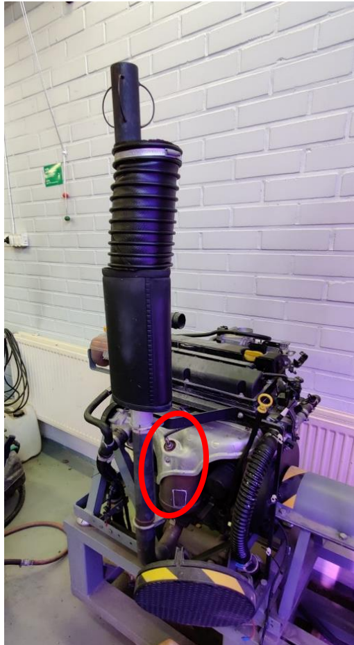
Figure 36. View of the catalytic converter of the Opel engine (Author's own).
