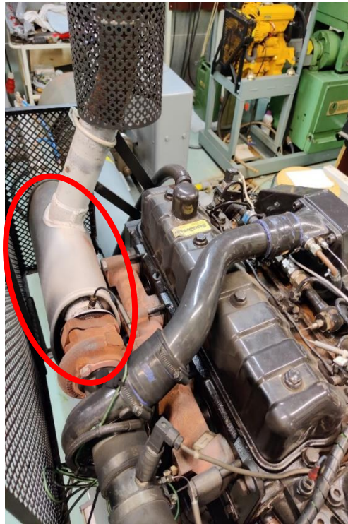
Figure 33. View of the exhaust manifold, turbo and muffler of the SISU engine with signalization of the muffler (Author's own).
