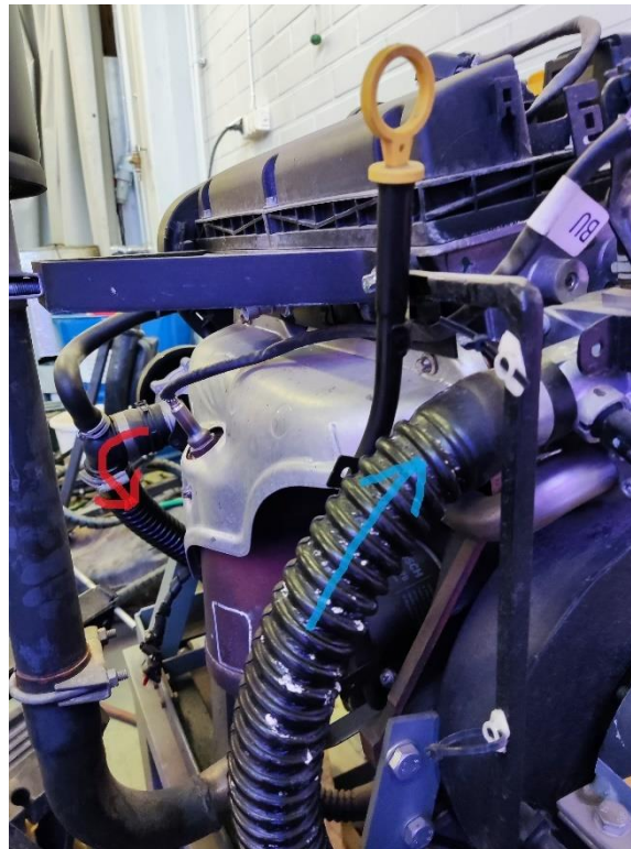
Figure 30. Inlet and outlet pipes for the coolant entering and leaving the engine block of the Opel motor (Author's own).
