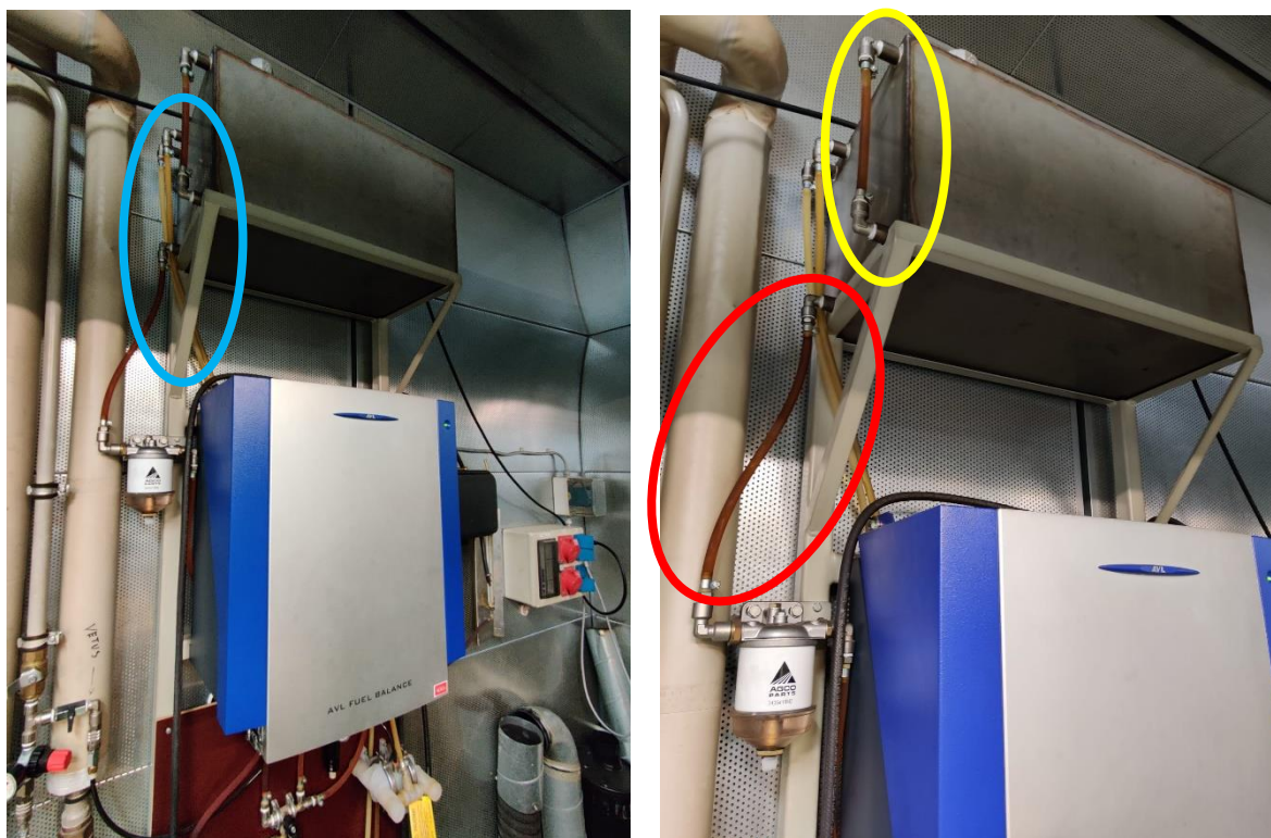
Figure 18 a) and b). Fuel tank used on the studied motor with indicators of the inlet (blue) and outlet pipes (red) (Author's own).
