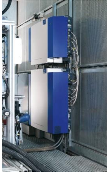
Figure 48. Mass Flow Meter and Fuel Temperature Control model AVL 735S /753C (AVL, 2021).
