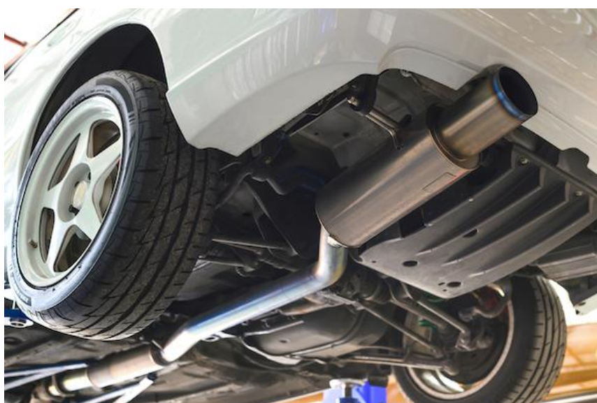
Figure 15. Tailpipe next to the muffler component in the back part of a car (Park Muffler, 2019).
