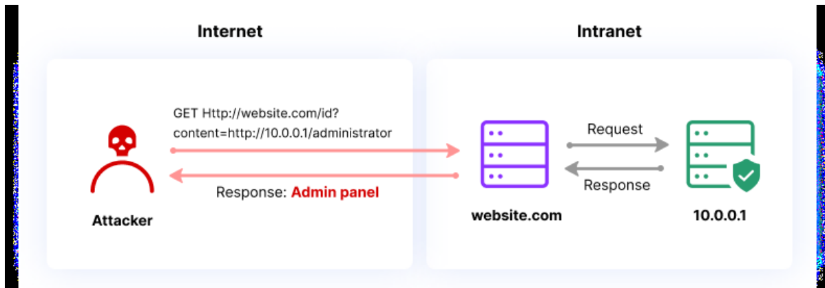
Figure 11. Attack scenario involving a SSRF attack (Imperva, 2019)
