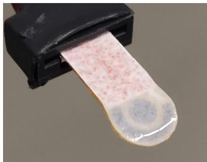
Picture 19. Paper sensor with the optimized measuring setup.
