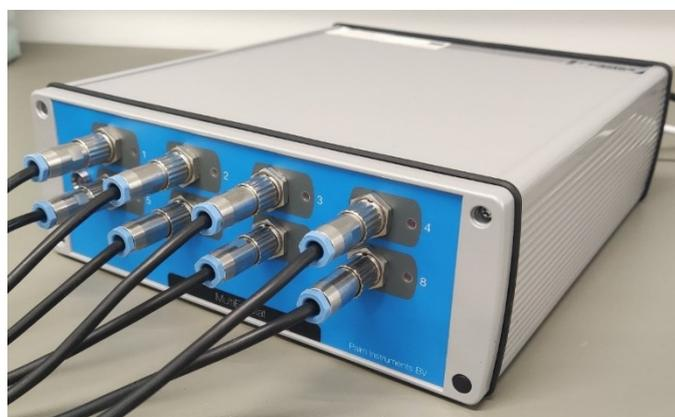
Picture 8. PalmSens 8-channel MultiEmStat2 potentiostat. Photo Credit: Niina Torniainen
