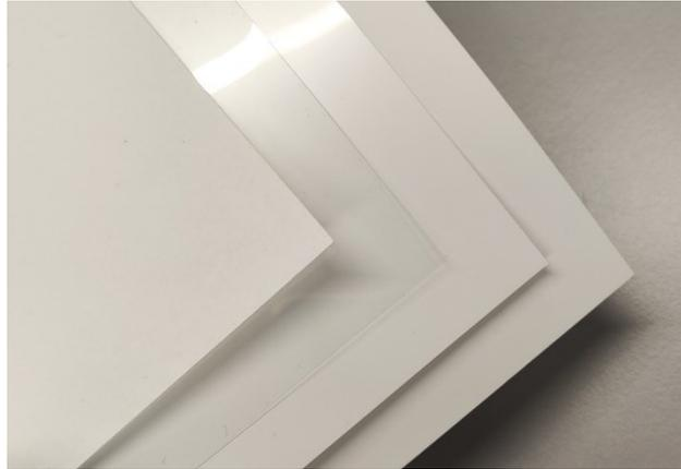
*Picture 3. Different substrates used for printing electrochemical sensors: paper, and PET with different surface treatments and transparency. Photo Credit: Niina Tornainen*
