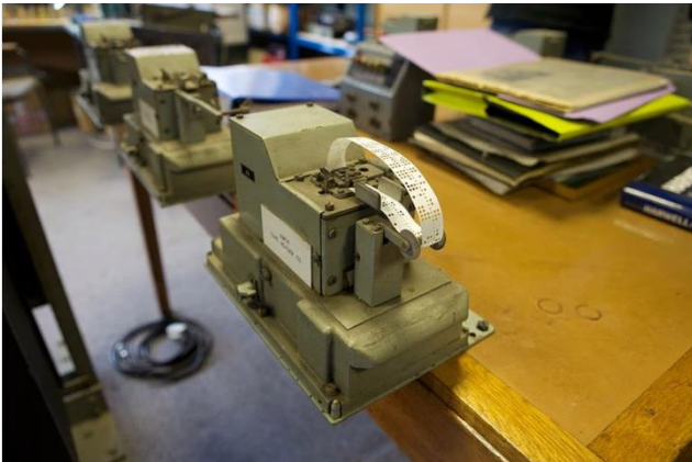
FIGURE 5. Paper tape reader on the Harwell computer (Bad Germ 2009)
