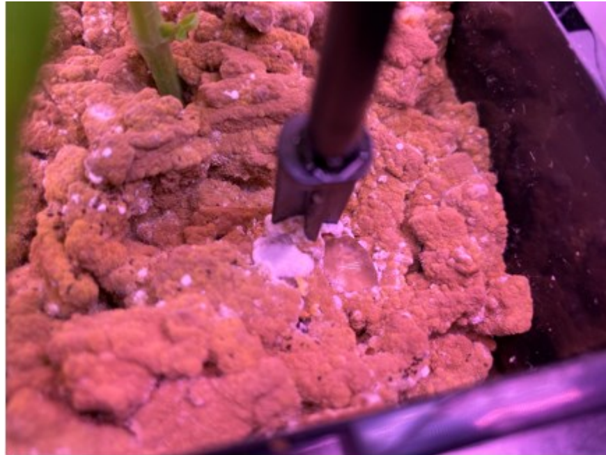
Figure 6. Cellulose fibres where mould prevents water from being absorbed by the substrate
