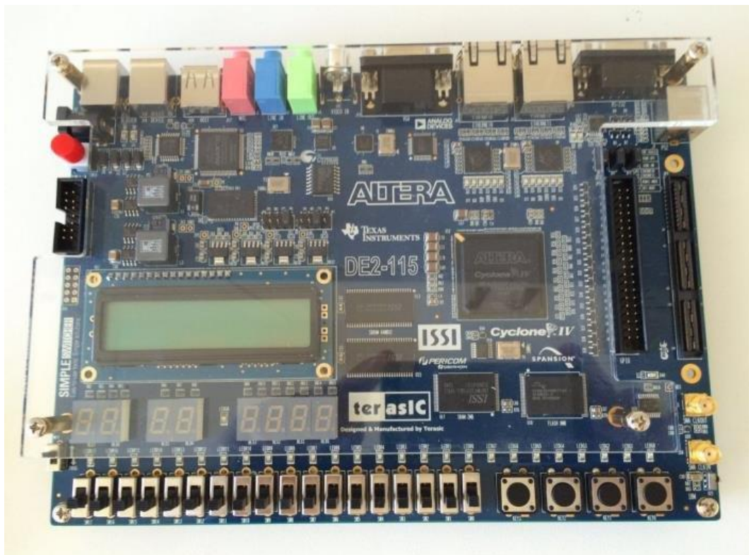
Figure 15. Altera DE2 board
