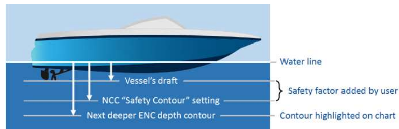
Figure 43 Example of how the Safety Contour is used in an ENC (NOAA, 2019)
