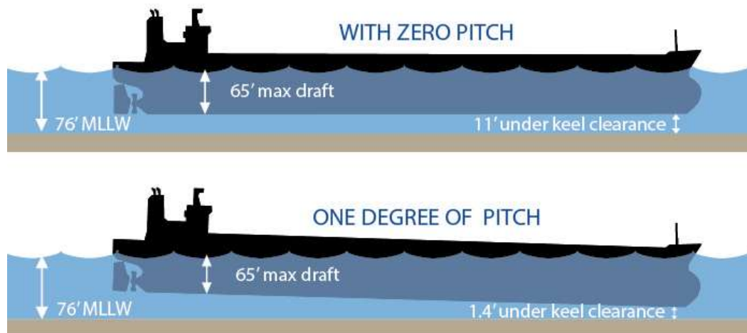
Figure 44 Potential pitch of a vessel entering the Port of Long Beach. (PORT OF LONG BEACH PRECISION NAVIGATION PROJECT, NOAA, 2017)
