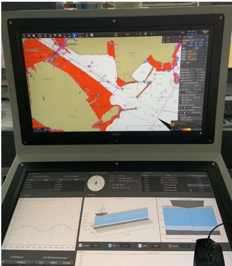
Figure 23 S-100 prototype ECDIS displaying S-101 electronic navigational chart in conjunction with S-129 Underkeel Clearance management data. (NOAA, 2019)
