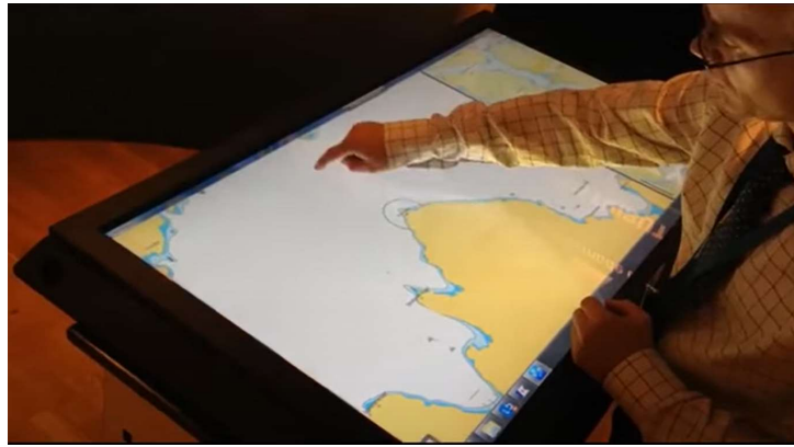
Figure 2 Using a touchscreen Back of Bridge Navigation software for planning routes (Navtor, 2015)
