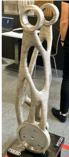
Figure 6. 3D printed replacement part for a robotic arm (Stevenson, 2019)
