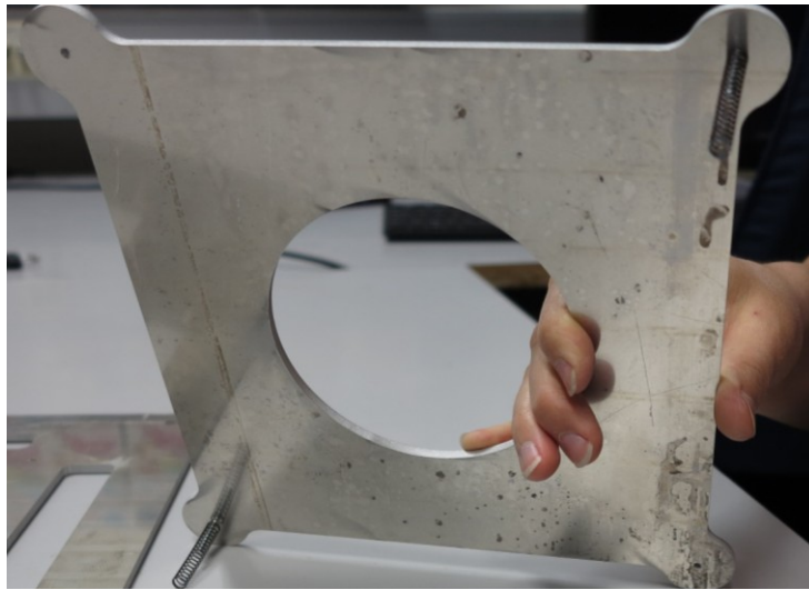
Figure 23. Springs inserted on the bolts
