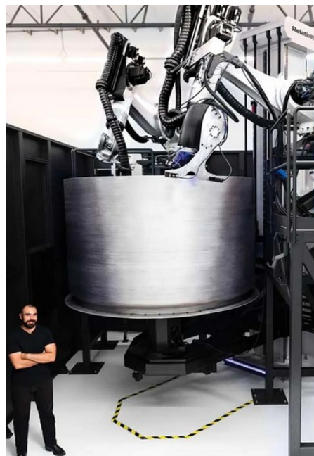
Figure 2. 3D printing a rocket (Relativity Space, n.d.)
