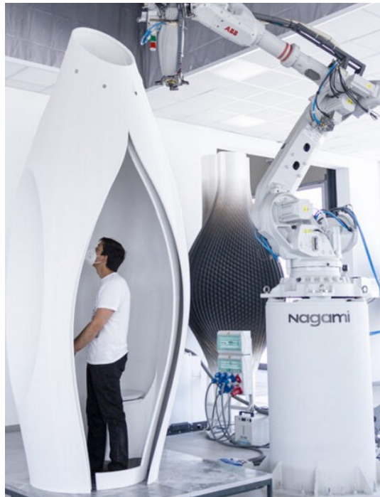
Figure 4. 3D printed portable toilet (Nagami, n.d.)
