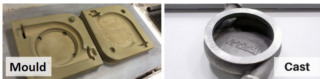
Figure 5. 3D printed sand casting mould (3HTi, n.d.)
