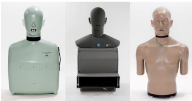
FIGURE 17. From left to right, Brüel & Kjær Type 4128-C, Head Acoustics HMS II.3 and G.R.A.S. KEMAR Type 45BM (Snaidero, Jacobsen & Buchholz 2011,30)
