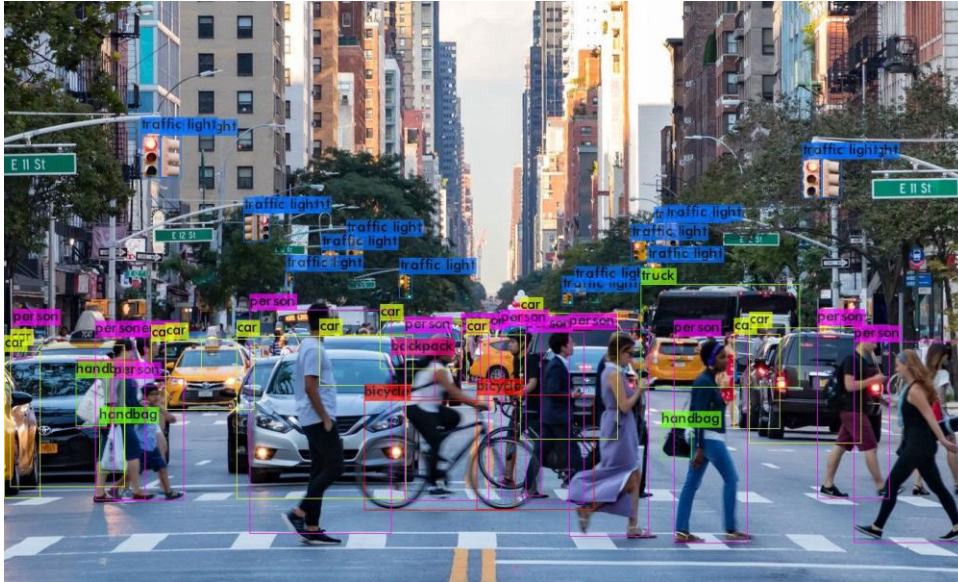
Figure 13. Object detection with YOLO4 [21].
