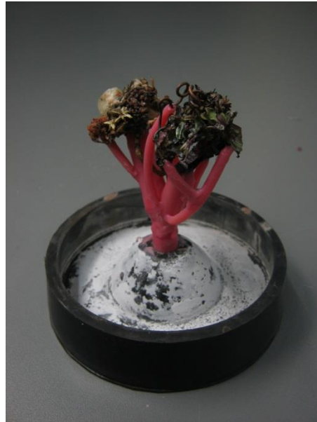
Figure 22. Example of prepared wax-tree for casting.
