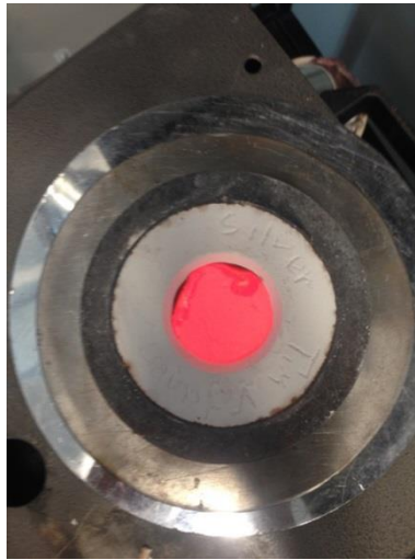
Figure 30. Flask with just poured hot metal.
