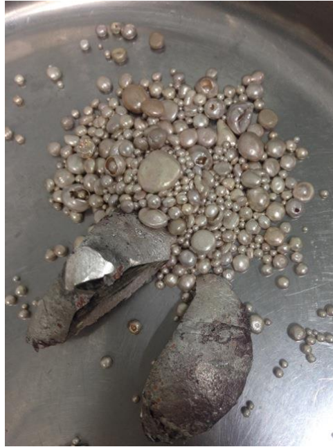
Figure 27. Preparing silver for casting
