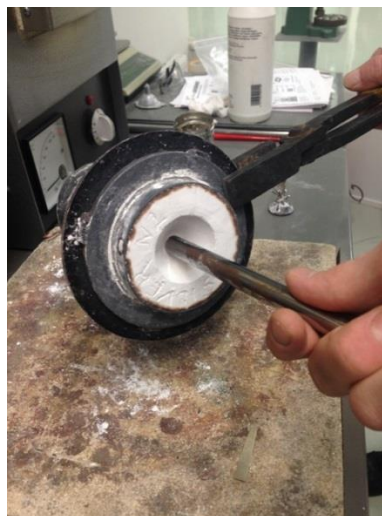
Figure 26. Applying vacuum cleaner, to get read of the ashes
