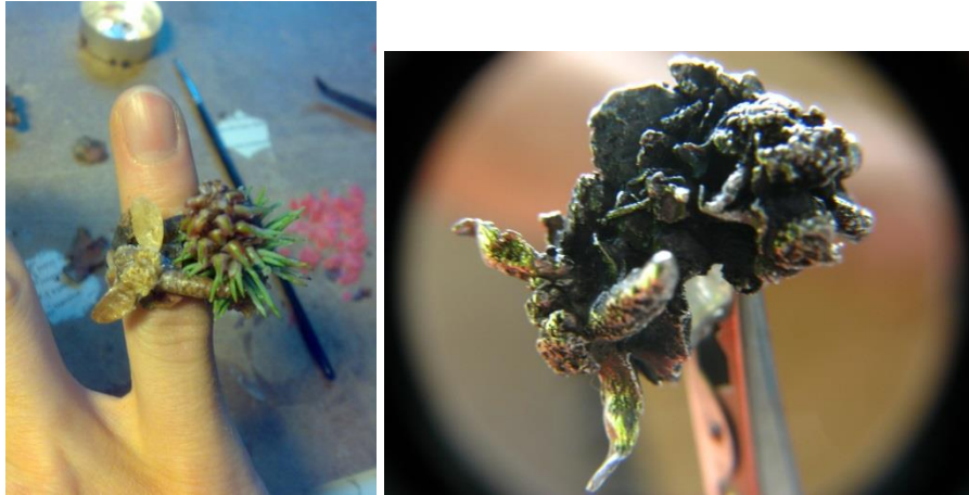
Figure 21. Example of wax/organic model, and the created piece.
