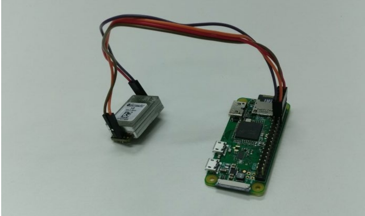
SBC and CO2 sensor connected together.
