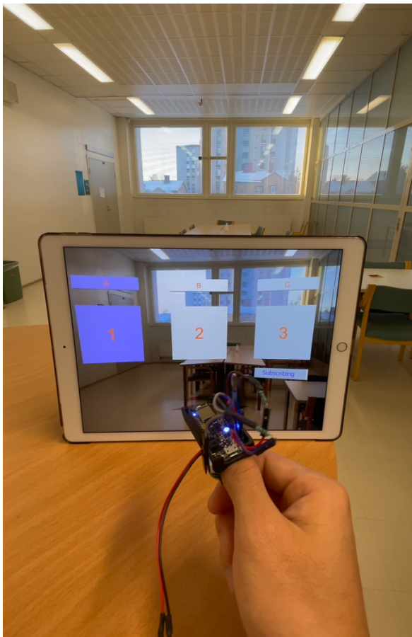
Figure 4. An AR application with the XR Controller
