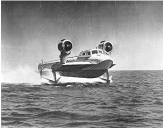
Figure 6. XCH-4 experimental hydrofoil (Unknown author, US Navy, 1950s)
