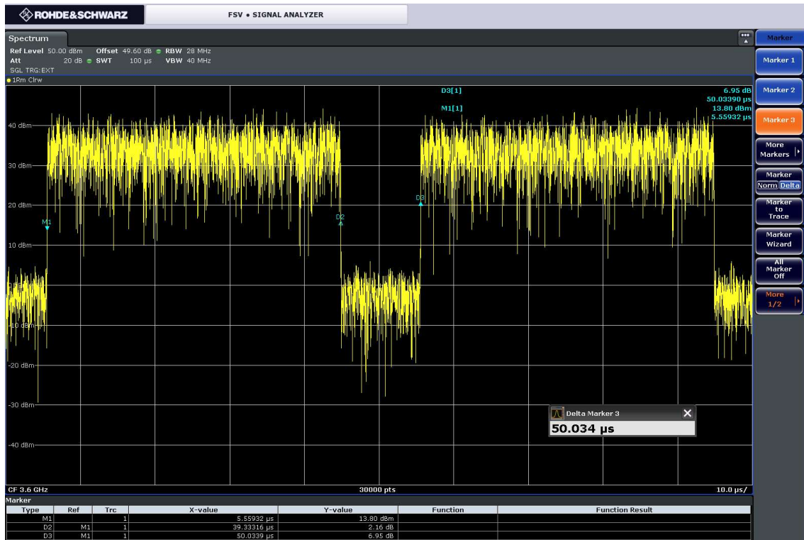
FIGURE 10. 50 µs long TDD signal in a signal analyzer
