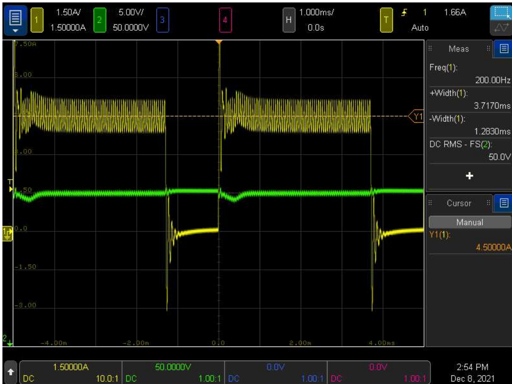
FIGURE 13. Current and voltage waveforms of 9 PAs with -0.5 dB gain target
