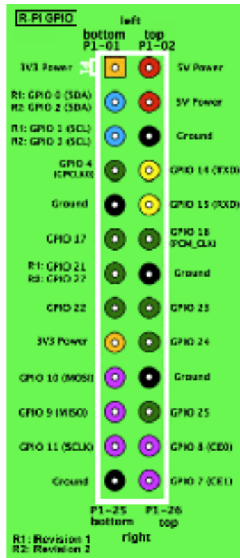
Figure 5: Raspberry Pi 2 GPIO (originally from eLinux.org).
