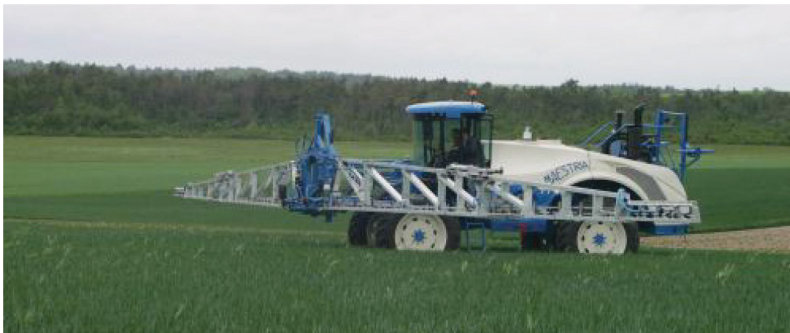
Figure 8. An example of aluminum spray boom in use. /17/
