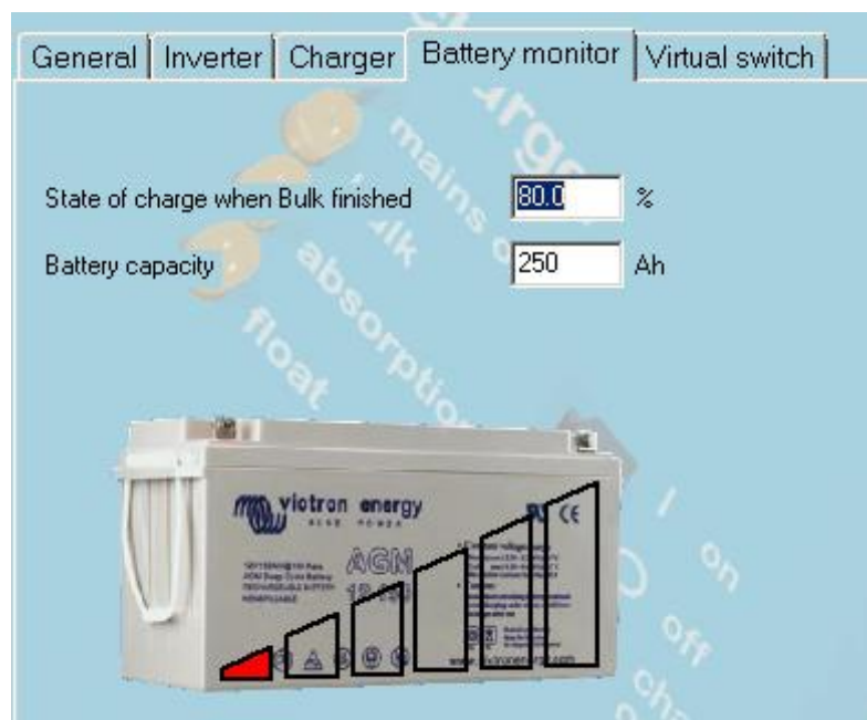
Figure 30 Battery monitor settings on the VE configure software TURKU UAS:BACHELOR'S THESIS | Constantino Miguélez Peña
