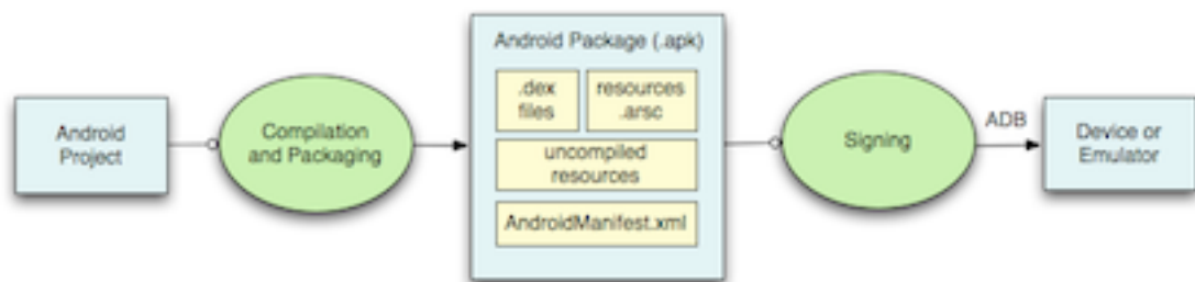
Figure 11. Android Compilation and Build Process
