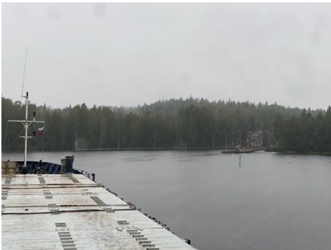
Figure 37: Ilistoe low-water approach at daylight. Plenty of space for maneuvering the approximately 70-degree turn into the lock. MV Nina inbound in the picture. (Antti Tasala, 2021)
