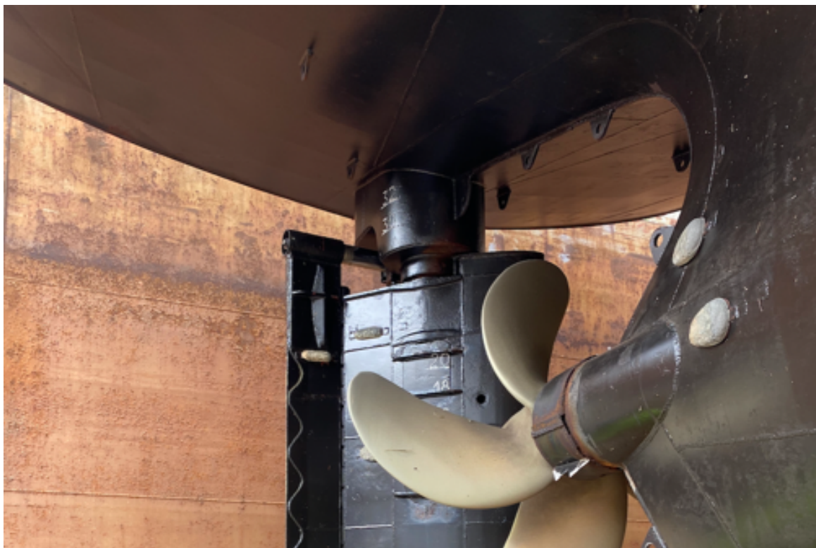
Figure 8: MV Nina's right-handed fixed pitch propeller and flap-rudder (Antti Tasala, 2020)
