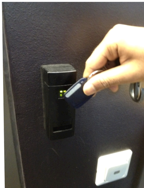
Figure 2: RFID reader and contactless key in practical use [Drawn by Author]
