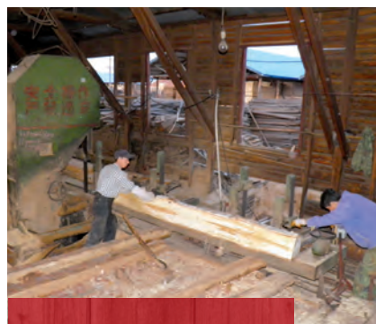
FIGURE 36. THE BAND SAW FOR DIVIDING THE LOG INTO LUMBER, GENHE
