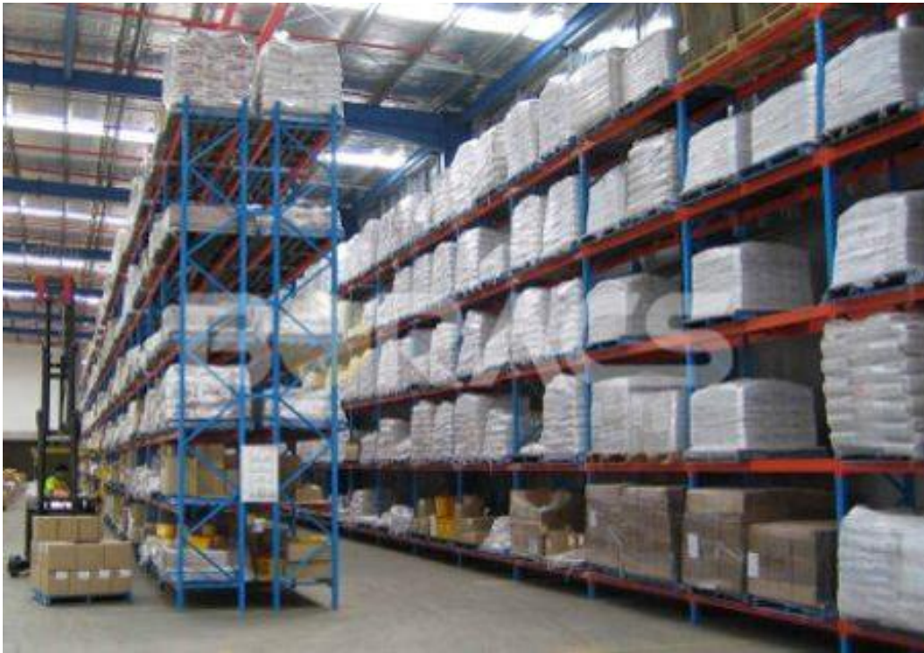
FIGURE 10. Selective pallet racks (BORACA LOGISTICS EQUIPMENT CO. LTD - Products Category. http://www.boracs.com/Products/Product_Category/ ).
