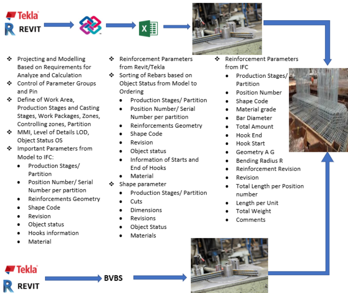
Figure 20: The required information in every stage and the lifecycle of the automated RFT fabrication from model to site (Jalali, 2018).
