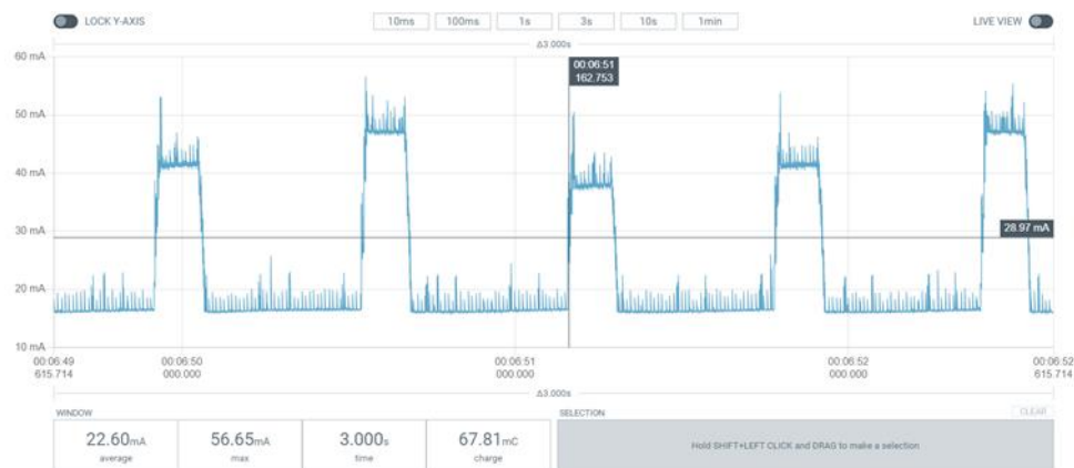
Figure 17. Figure 14. A screen capture of the PPK, that shows the current consumption of the DUT with all chips active and the RGB LEDs flashing with power management enabled.
