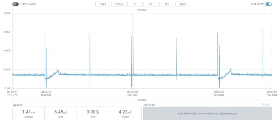
Figure 16. A screen capture from the PPK that illustrates the current consumed by the DUT with a capacitive touch sensor in a full power mode, with a custom power management implementation (the sensor is rated to consume 0.9 mA in this mode).
