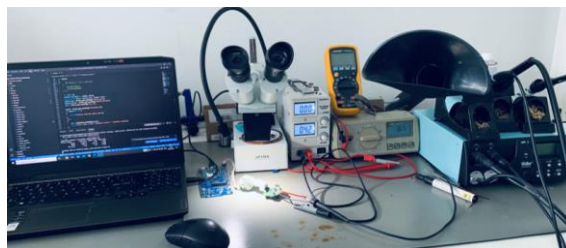
Picture 4. Workshop tools and equipment, with the DUT connected to a DMM in series with a power supply.
