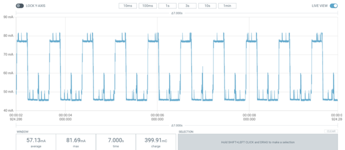
Figure 14. A screen capture of the PPK, that shows the current consumption of the DUT with all chips active and the RGB LEDs flashing without any power management enabled.
