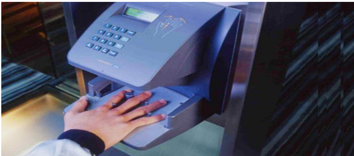
Figure 24. An individual with hand placed on hand geometry reader scanning platen (Thakkar, n.d.).
