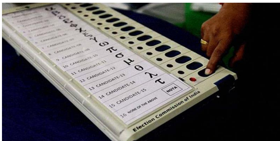
Figure 15. An electronic voting machine in use while in an election in India (Thakkar, n.d.).
