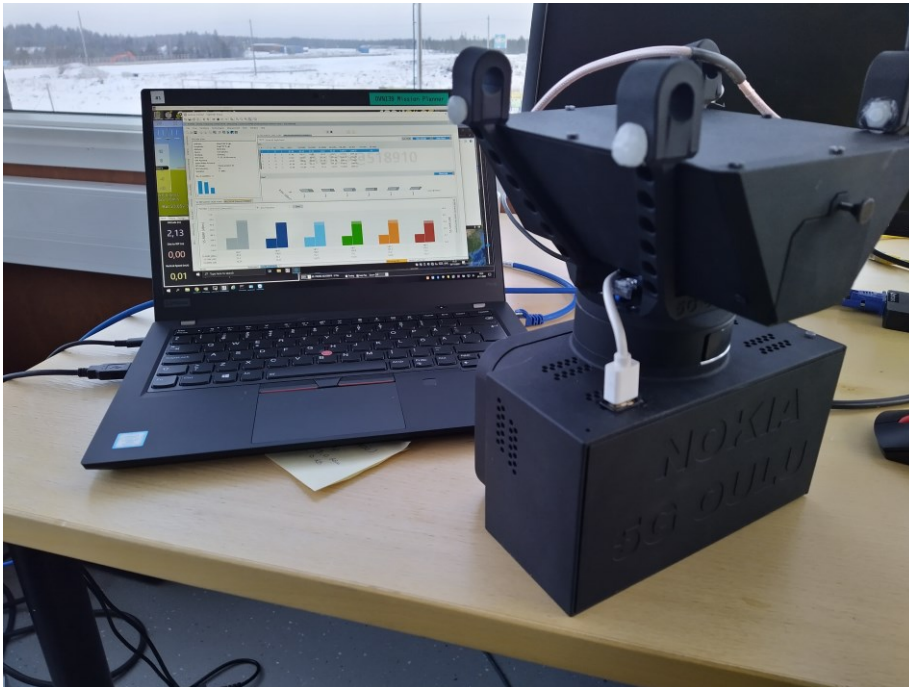
FIGURE 13. R&S ROMES4 software, payload adapter and 5G MABS
