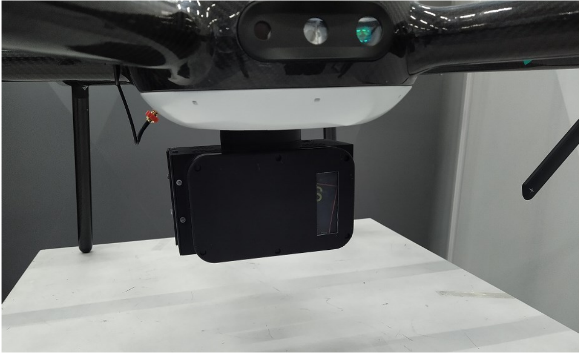
FIGURE 6. 5G MABS attached to Nokia drone
