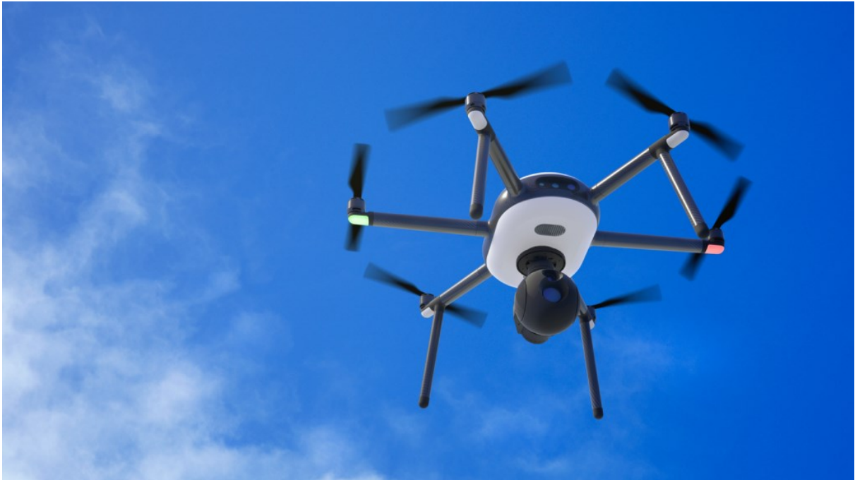
FIGURE 12. Nokia drone with camera gimbal payload [8]
