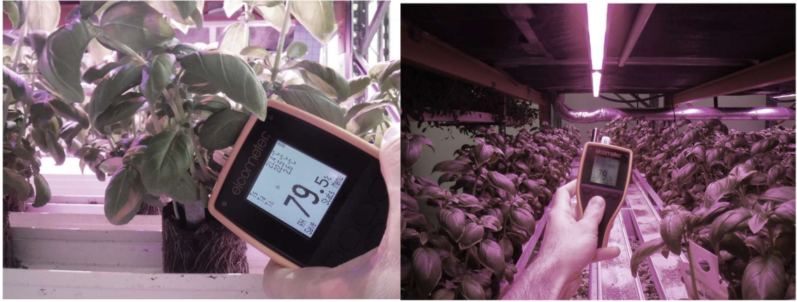
PICTURE 2. Handheld Elcometer 319 Dew Point measurement examples. Left: Elcometer measuring air temperature and RH% within the plant canopy, Right: Elcometer measuring air temperature and RH% above the canopy within the module (Denham 2021)
