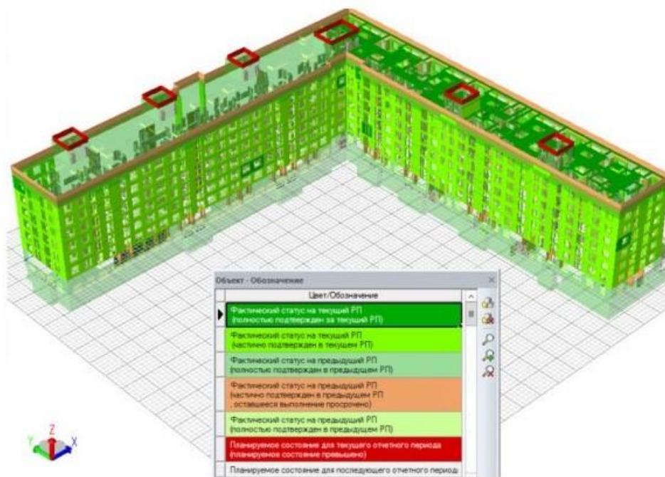
Figure 3.17 Indication of completed work on a 3D model in ITWO (project "Inkeri", Pushkin) (Maltsev 2019, 147)
