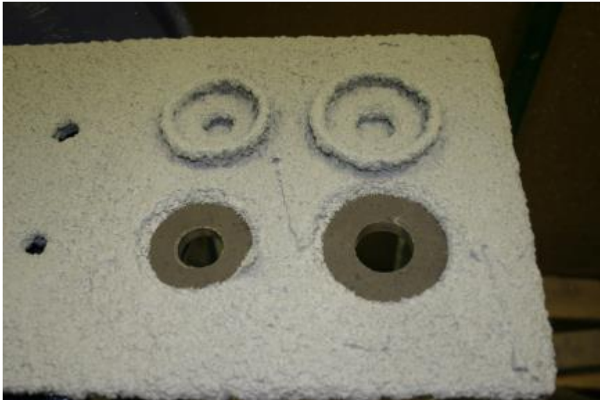
Figure 6. Masking bungs to avoid problem with bolt tightening (AkzoNobel, n.d.)
