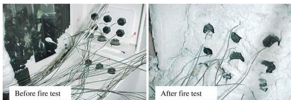
Figure 9. Fire test with fully protected steel joint and unprotected bolts assembly (Dai, Wang, & Bailey, 2010, p. 29)
