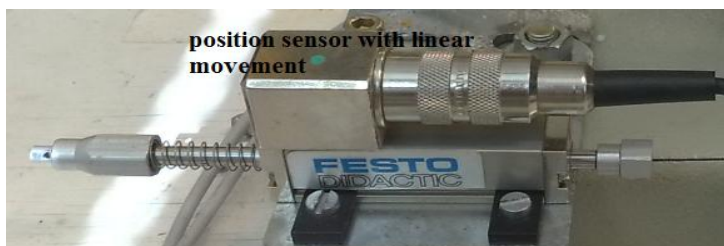
Figure 12 position meter sensor
