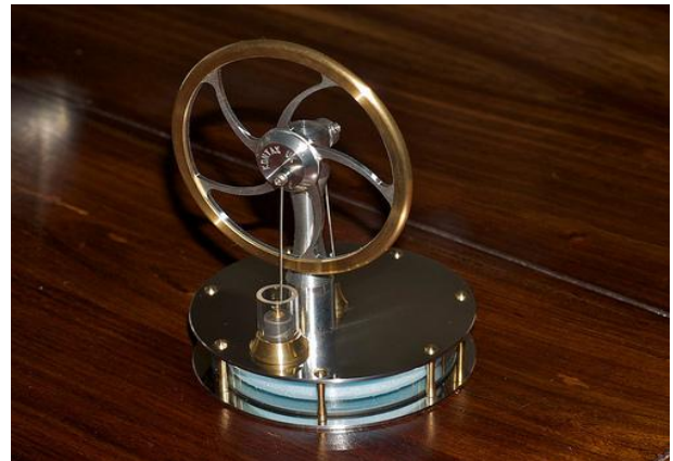
Figure1 Modern Stirling engine
