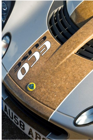
Figure 6. Lotus Eco Elise with organic hemp fibre composite [17].
