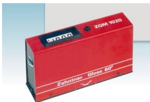
Figure 34. Gloss measuring device [49].
