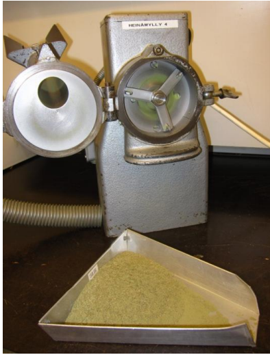
PICTURE 3. Cyclonic mill and the dried, ground grass biomass ready for analyzes.
