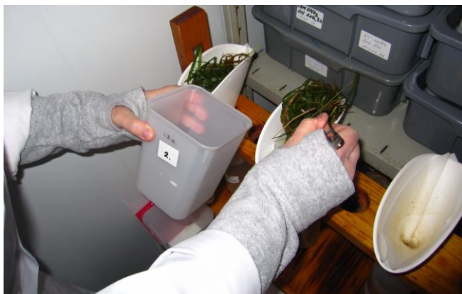
PICTURE 6. The water and grass biomass material was separated through filtration paper and the biomass was collected back to freezing box and frozen.
