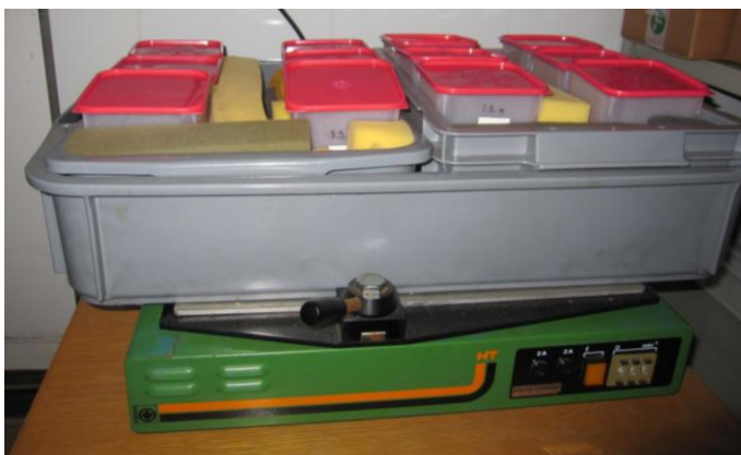
PICTURE 4. After adding deionised water (400 ml) to the thawed grass biomass, the boxes were placed in a reciprocating shaker (run at 200 rpm for an hour).
