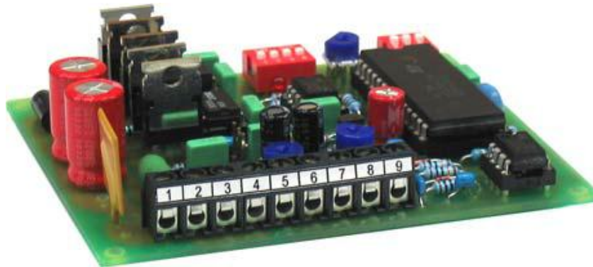
Figure 6.3 DC Motor Controller
