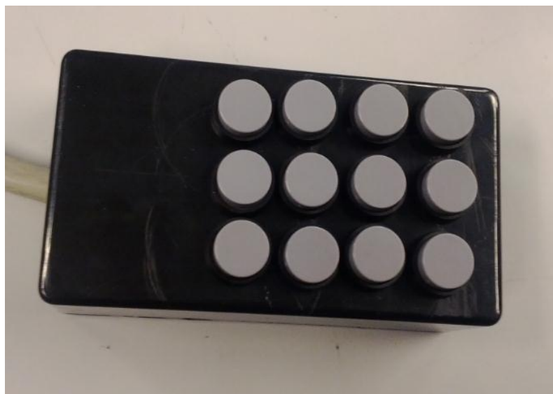
Figure 6.7 Control pendent for controlling the movements of the Robotic Arm
