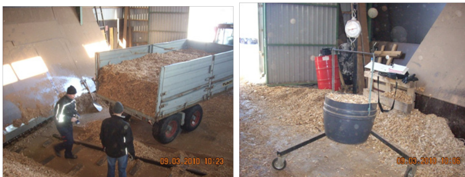
Figure 3.3. Delivery of chips by tractor and loose density calculation. Photo: Martti Härkönen
