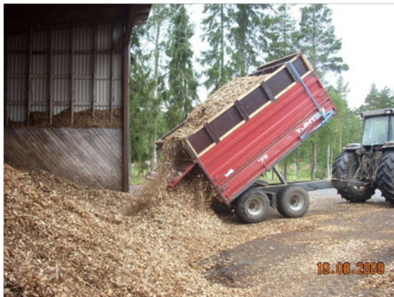
Figure 2.6. A load of green woodchips arriving at a heating plant. Load volume is 10 \text{ i-m}^3 . What is the mass of the woodchips in the load? Photo: Martti Härkönen
