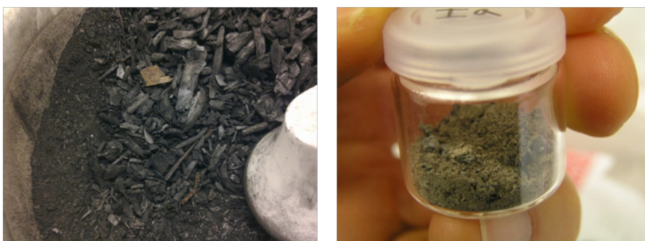
Figure 3.6. Laboratory analysis of dry matter in ash samples. Photos: Anu-Sisko Perttunen
