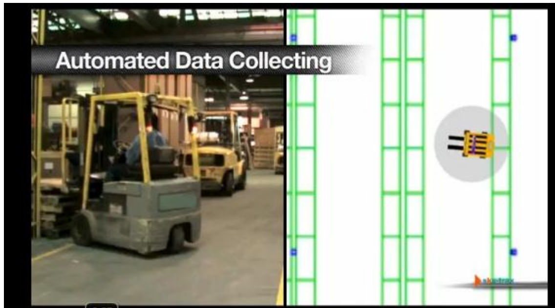
GRAPH 17. Vehicle tracking system using 2D barcodes (Sky-Trax Incorporated 2012.)
