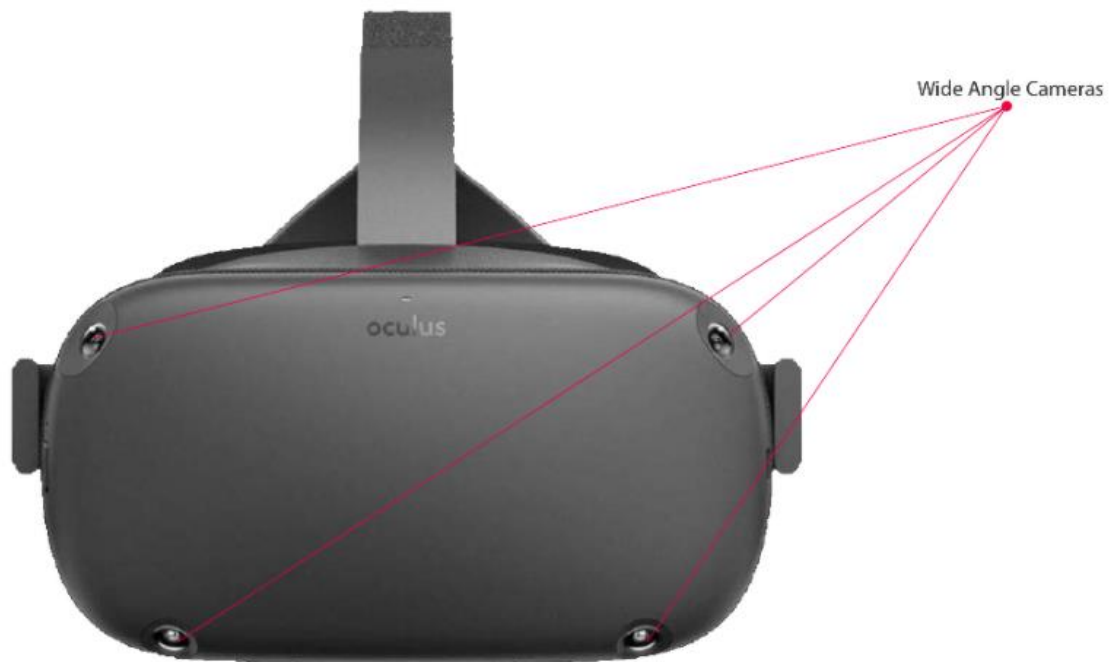
Picture 2. Oculus Quest hand tracking cameras. [15]
