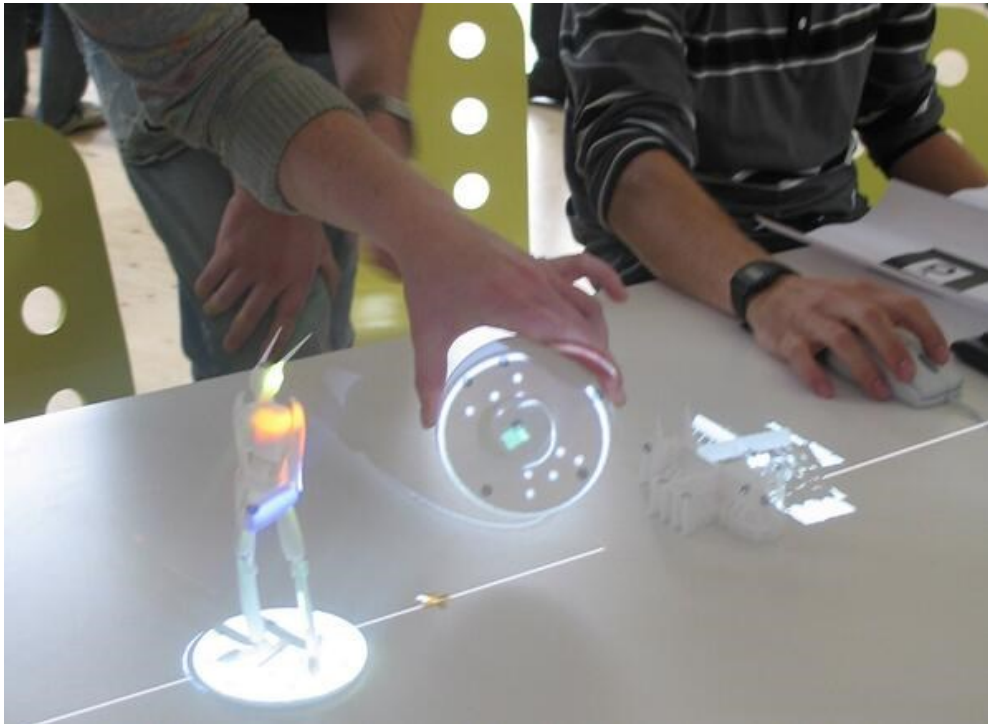
Figure 5. 3D objects are displayed by projecting light on a table (Poetker, 2019)
