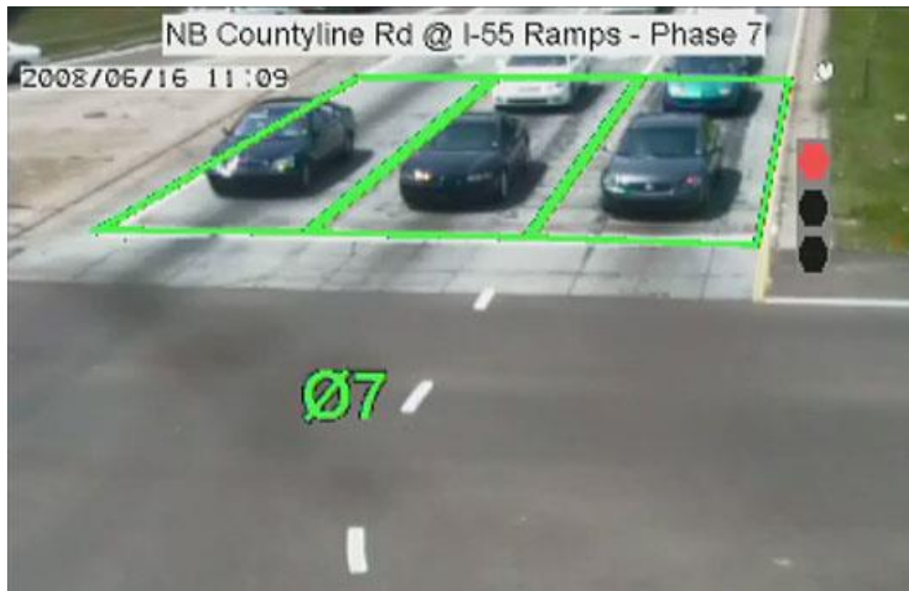
Figure 3 Possible placement of video detection at an intersection (Hanson, 2017)
