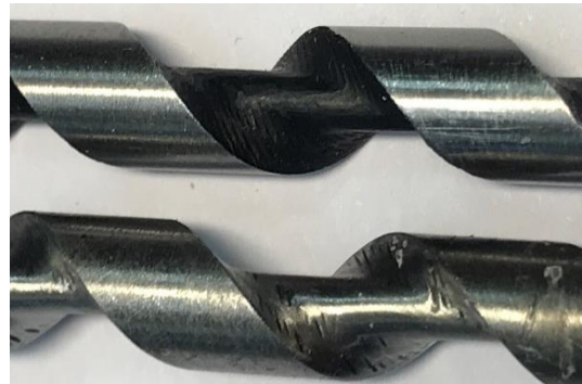
Figure 21. Comparison of pre and post sanding of the screw
