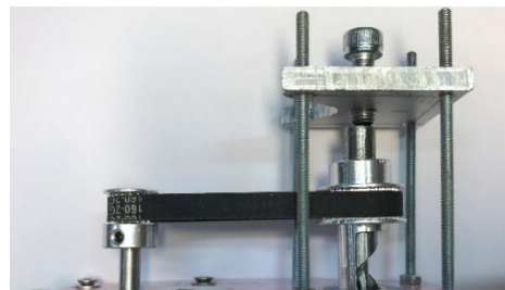
Figure 23. Tensioning plate mounted
