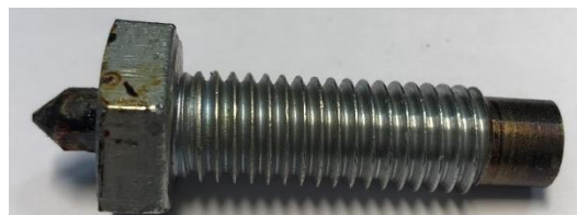
Figure 19. Drilled out bolt and nozzle
