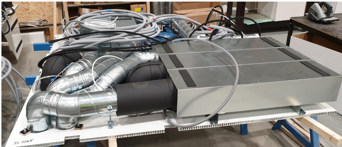
Figure 16: Ventilation equipment assembly.
