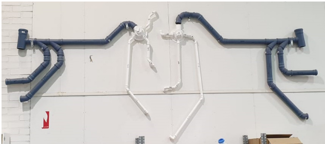
Figure 14: Drainage layout at the prefabrication factory.
