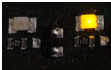
Figure 55. LED with a 5% pulse width
