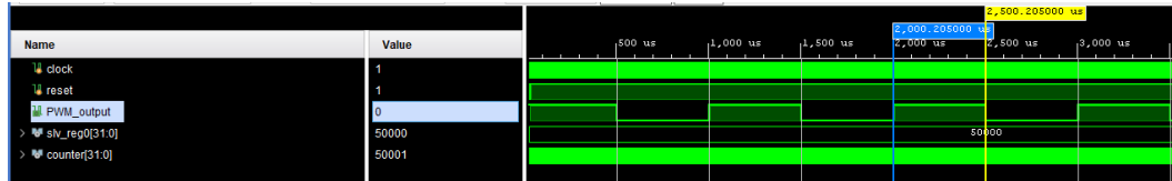
Figure 41. Simulation with 50% pulse width
