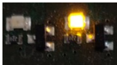
Figure 54. LED with a 35% pulse width
