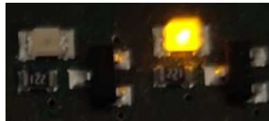
Figure 73. Pulse width of 25% on the LED
