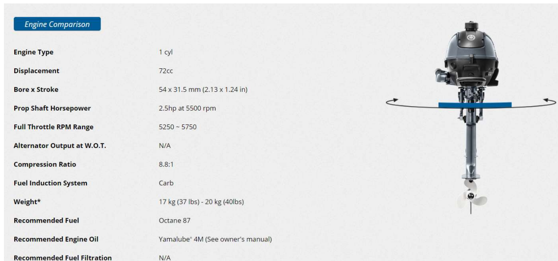
Figure 5. Yamaha 2.5 hp outboard specifications (Yamaha Outboards, 2020)
