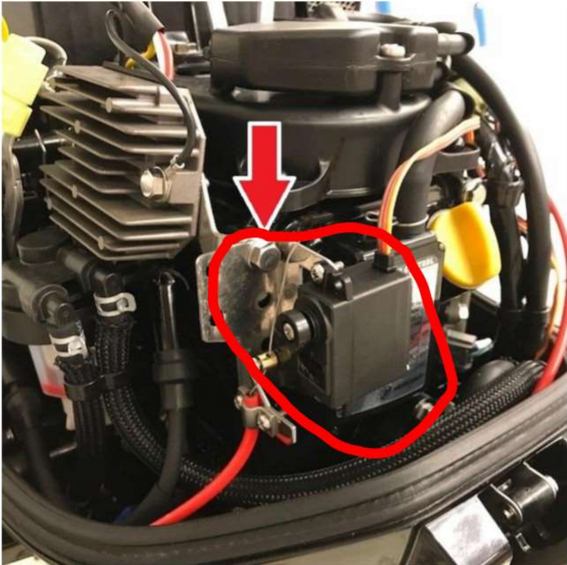
Figure 6. Wireless throttle control (TROLLMaster 2020, n.d.)
