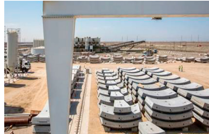
Figure 2.11 Precast Segment rings with diameter of 12.60 m under Suez Canal (Author)
