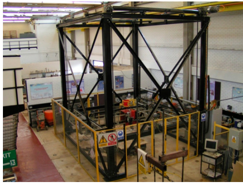
Figure 20 The printing frame of Concrete Printing
