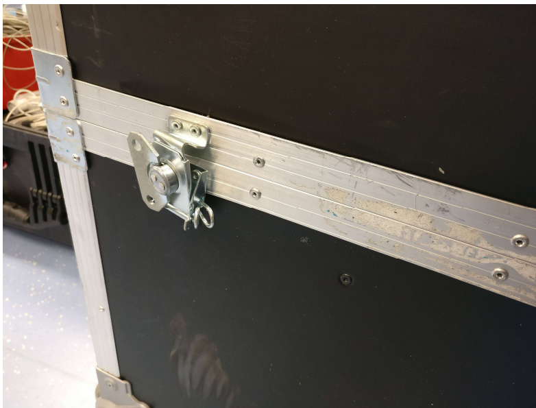
Figure 5 Ametek case locks damaged in use
