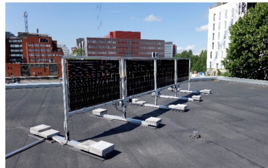
Fig. 1: Bifacial EWV test setup on the rooftop of the TUAS facility in Turku Finland (60°N). Apartment buildings generate some late evening shading for test system during the summer months.
