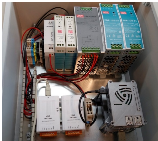
Fig. 3: Data collection system with two Raspberry Pi minicomputers and redundant power supplies.
