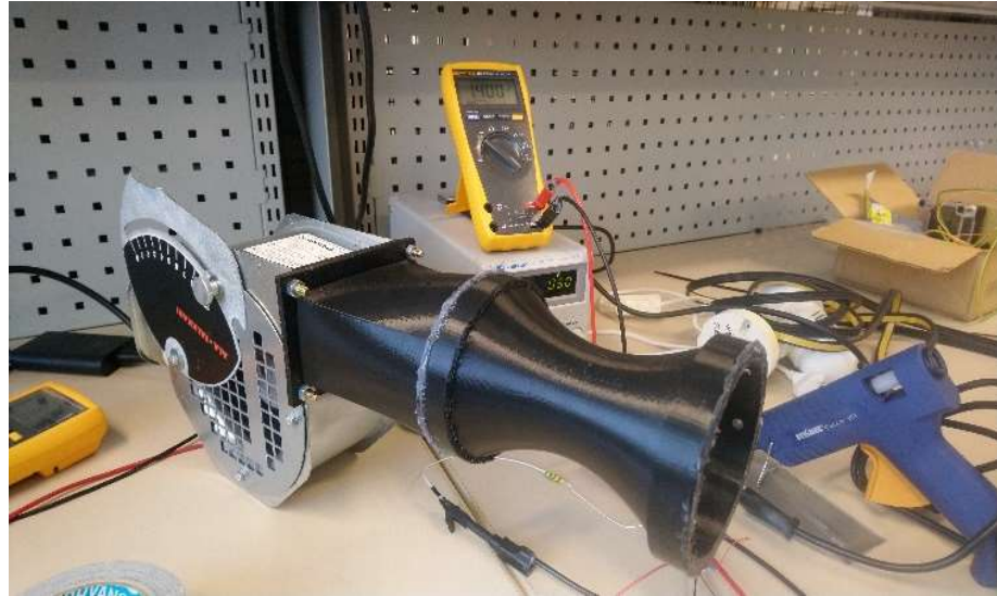
Figure 8. Venturi turbulence test station
