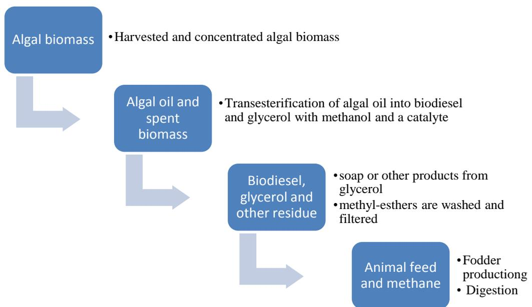
Figure 1: Microalgal biodiesel refinery: producing multiple products (information adapted from Oilgae 2010)
