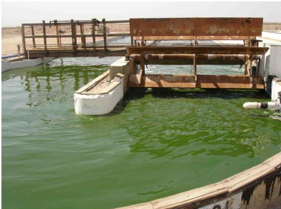
Figure 3: Paddle-wheel of a raceway pond (Oilgae 2011)
