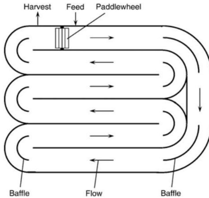
Figure 2: Aerial view of a raceway pond (Chisti, Y. 2007)
